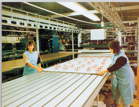
the finished lay package is fixed by the VEITH Needle Plates
