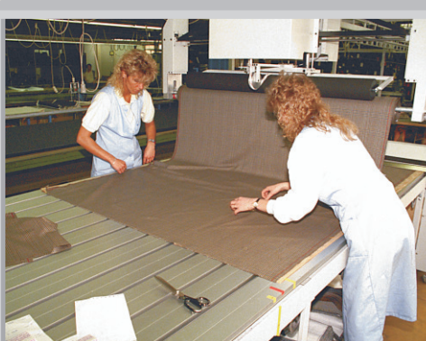
spreading the fabric and matching it in one step
