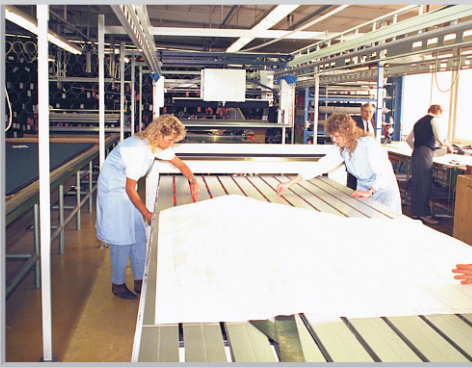
the needle bars are positioned according to the marker
