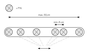
The dimensions of the table for the **VEITH SYSTEM** Linear Matching Device are as follows:
